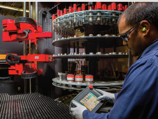
With 220 punches and 440 dies, the PDC ensures that the right tool is always available.
